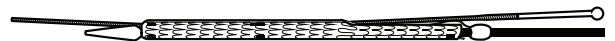
Figure 3C: Constrained IBC on Delivery Catheter with Radiopaque Markers and Removeable Guidewire Tube (RGT)
